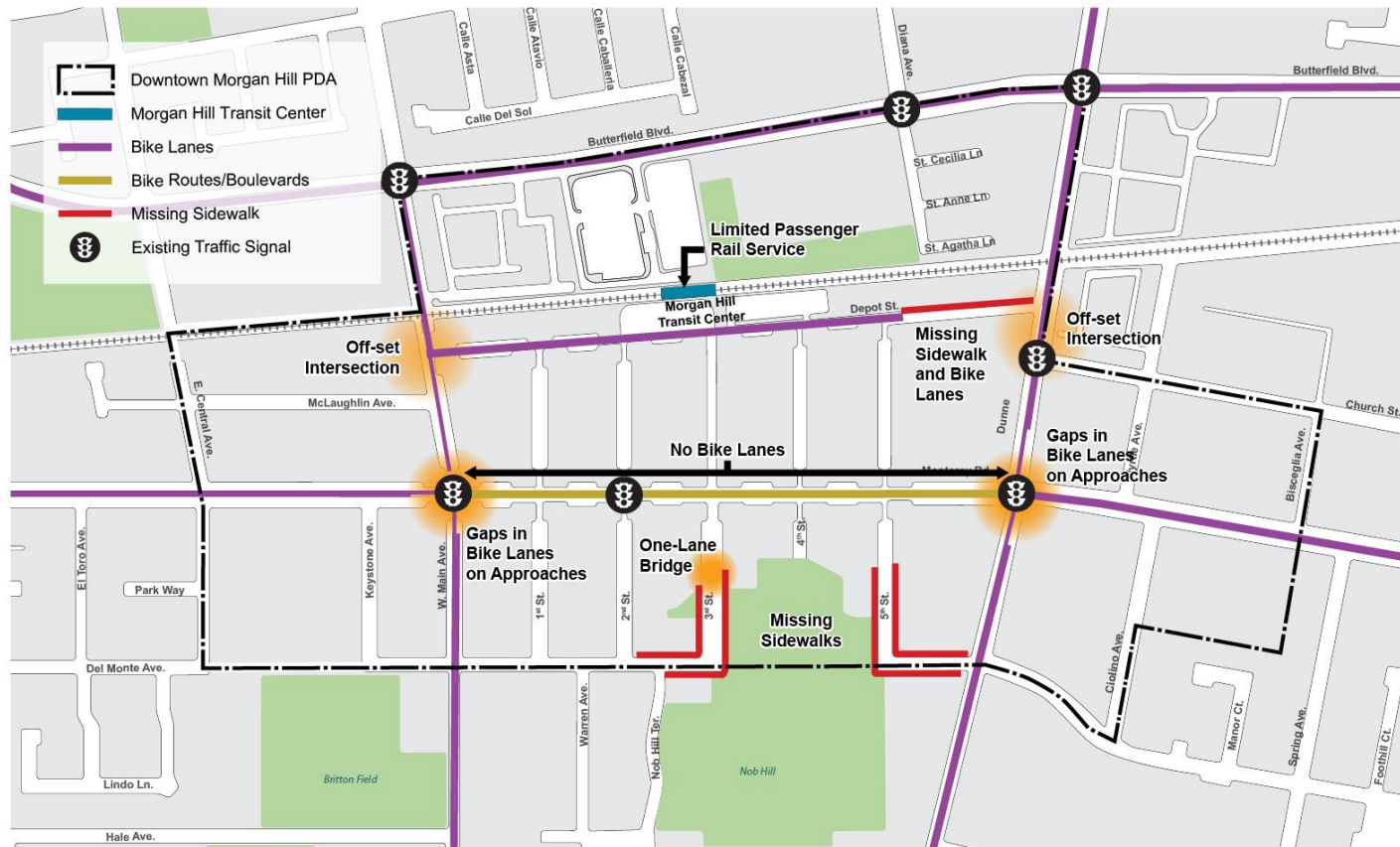
Figure 3-1: Gaps in Existing Transportation System
