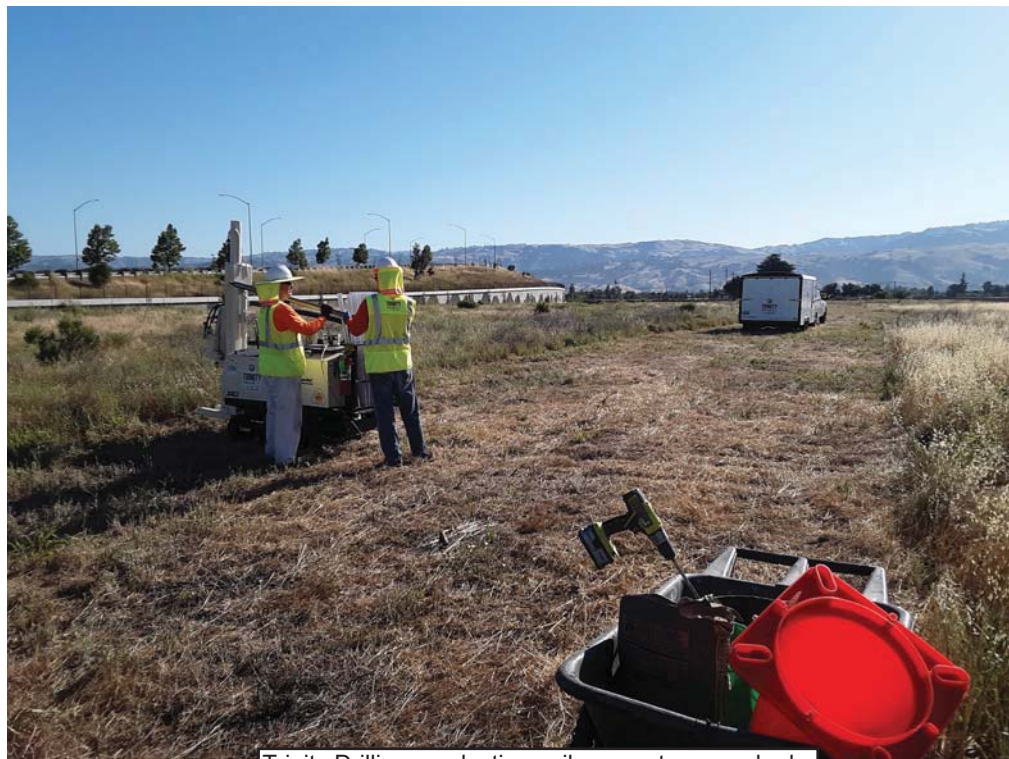
Trinity Drilling conducting soil cores at pre-marked locations with hydraulic driven probe track rig.
