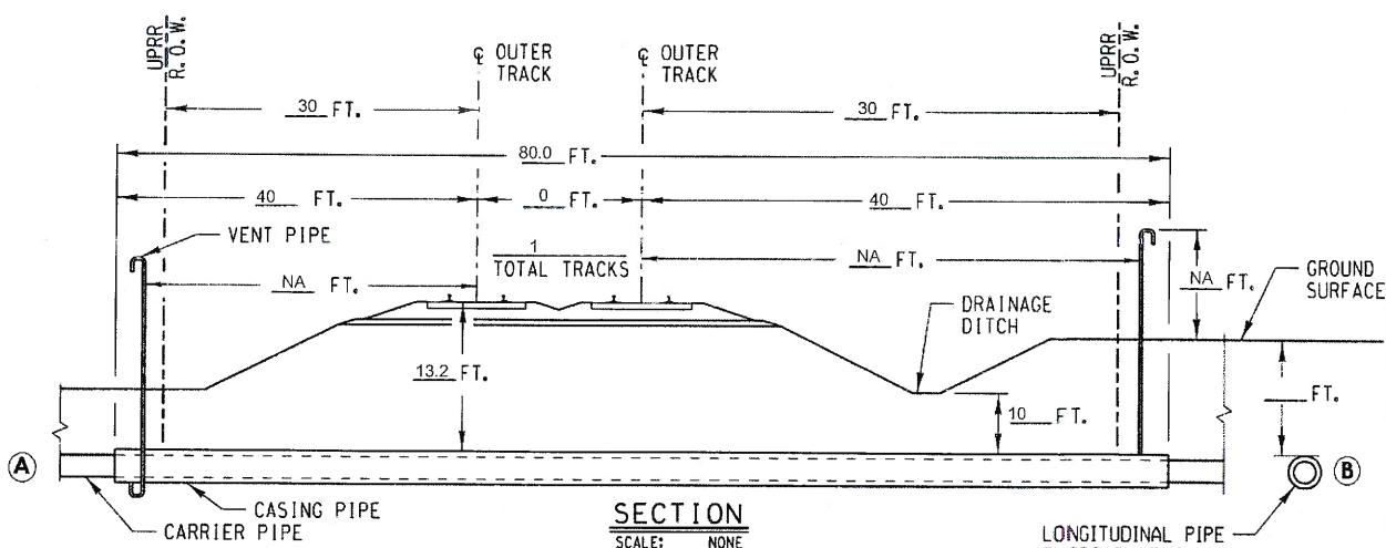
NOTES: See Exhibit A-1 for additional details about this pipe ties in with an existing SS pipeline encroachment running parallel to and north of UP track.
