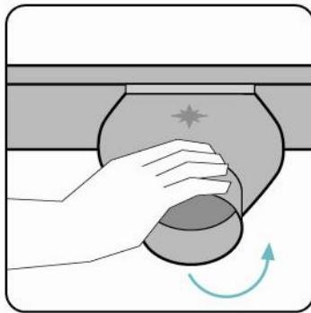
**Step 2:** Bend the clips (first the left, and then the right) to the top of the back flange of the gutter to fasten outlet, and move to Step 3.
