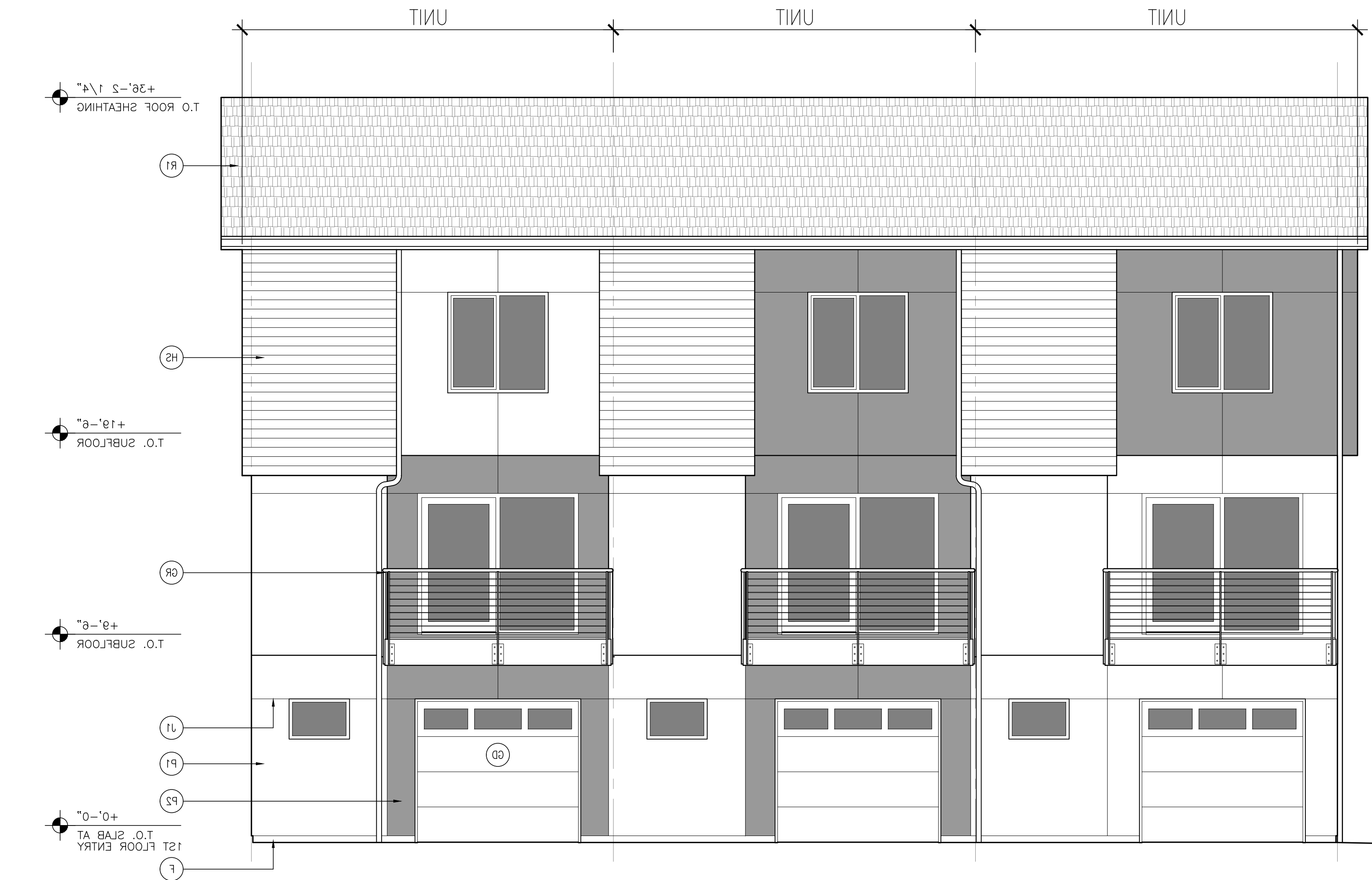
BUILDING 2 - SOUTH ELEVATION
