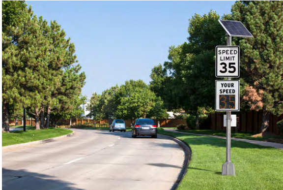
FIGURE 52 Pole-mounted Radar-Speed Sign (Source: Tim Magee)
